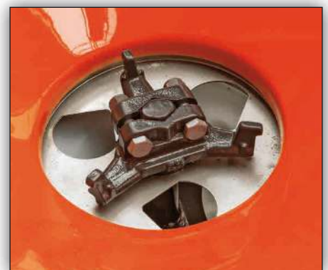
Agitator ensures even feed of the fertiliser
