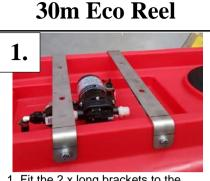
1. Fit the 2 x long brackets to the tank with 4x M8x16mm Bolts, Washer & Spring Washers
